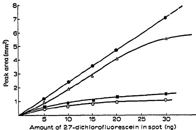
Fig. 4. Change of linearity due to change in exciting wavelength. ●, 310 nm; △, 300 nm; ■, 320 nm; ○, 290 nm. (From Touchstone et al. 8 , reproduced with permission of the authors and the American Chemical Society.)
